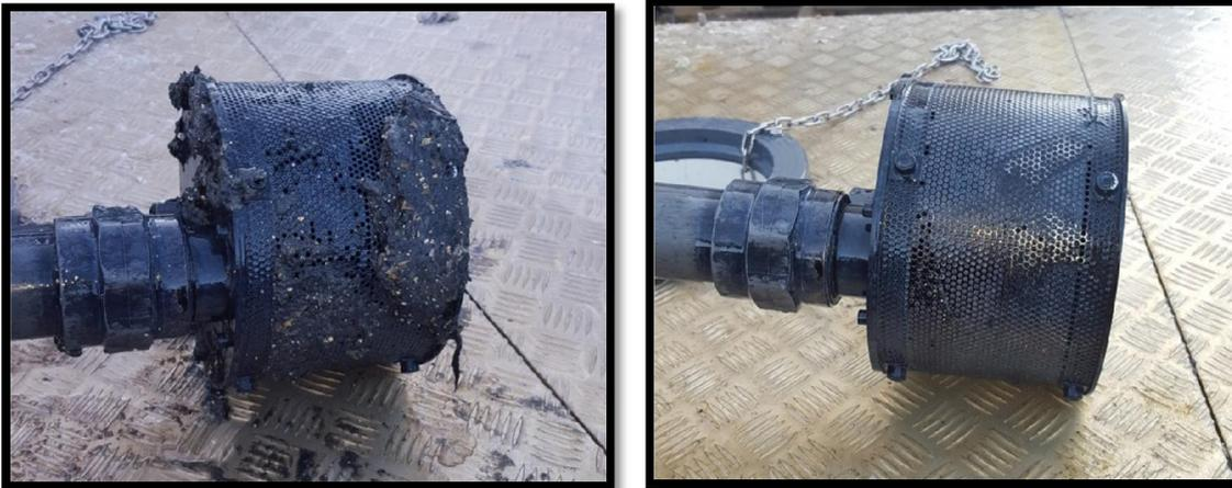
Figure 2 : Rotorflush RF200R straight from service (L) and after low pressure wash down (R)
