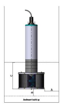
A.300mm min gap to side of tank (600mm between two filterpumps)
