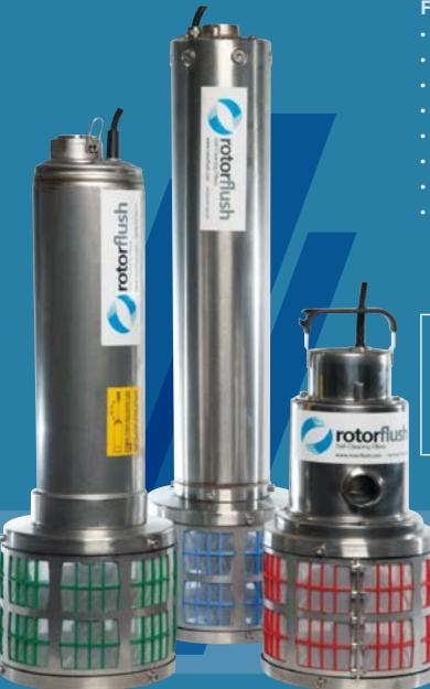
The self-cleaning inlet filters are capable of filtering from 40 to 660 US GPM. They have screen apertures ranging from 230 mesh – 45 mesh on the fine filters, and 35 mesh - 3 mesh for coarser filtration. They protect the pump and other equipment from blockage. They extend pump life and reduce maintenance to a minimum.
